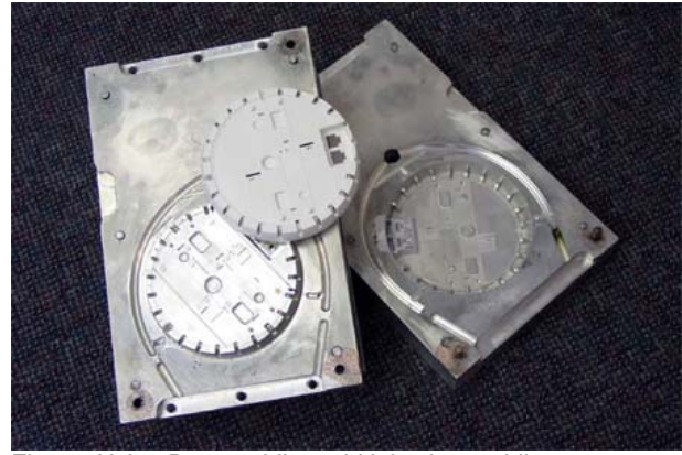
Fig. 2 - Using Protomold's rapid injection molding process, Trapeze skipped rapid prototyping and went directly to functional testing and production ramp-up of its Mobility Point housing. The Trapeze Networks™ Mobility Point is a system device that augmen
