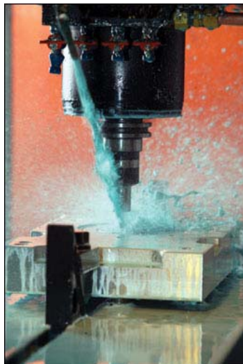
In rapid injection molding, the 3D CAD file used to generate the mold design is downloaded into Protomold's software system, which then automatically outputs tool paths for the high-speed HAAS CNC machine centers to manufacture the molds.
