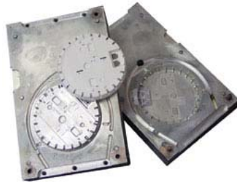
Trapeze skipped rapid prototyping and went directly to functional testing and production ramp-up of its Mobility Point housing, shown here with its mold.
